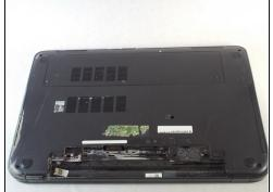
Use your thumb to lift the battery out of its slot by lifting the bottom edge of the battery.
