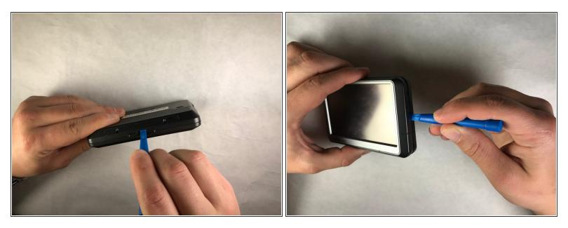
Once screws are removed, use the plastic opening tool to carefully separate the body from the screen encasing.
