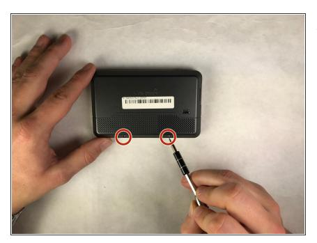
Remove two 4mm T5 Torx screws located under the sticker.
