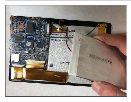
• Remove your old battery and replace it with the new battery.
