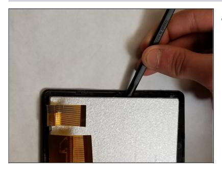
• Insert the plastic spudger underneath the screen display and lift.
