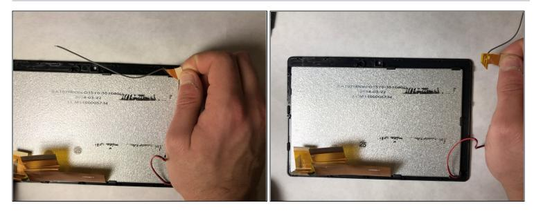
• Remove the grey wire from the back of the screen display.
