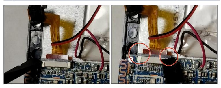
• Use the plastic spudger to pry the tabs open on the digitizer ribbon sockets.
