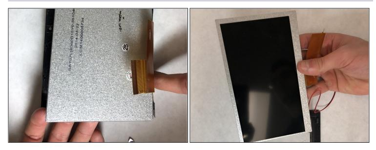
• Continue lifting the screen by hand and pull it out until it is completely removed.
