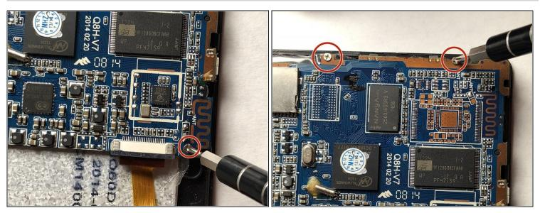
• Unscrew the motherboard from the screen with the JIS #000 Screwdriver, a Phillipshead type screwdriver
