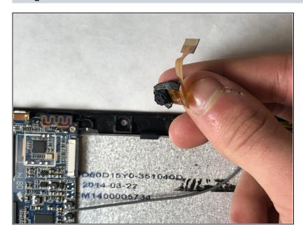
• Pull the camera out of the device.
