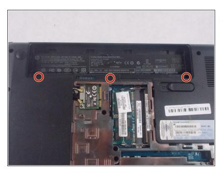
Remove 3 screws located where the battery previously was.
