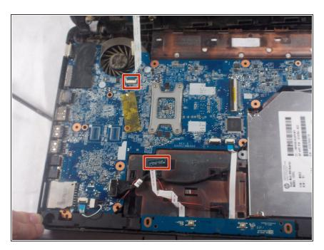
Unplug wires connecting back panel to keyboard.
