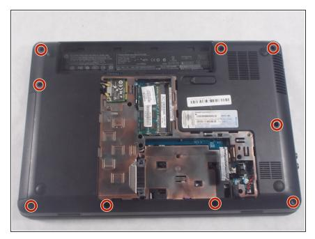
Unscrew all nine 6.0mm JIS #0 screws located on the border of the back panel.
