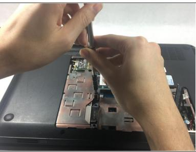
Remove 6 screws located under the spot where the smaller L-shaped panel was located.
