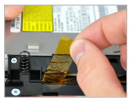
If necessary, remove the yellow kapton tape covering the internal frame and the optical drive.
