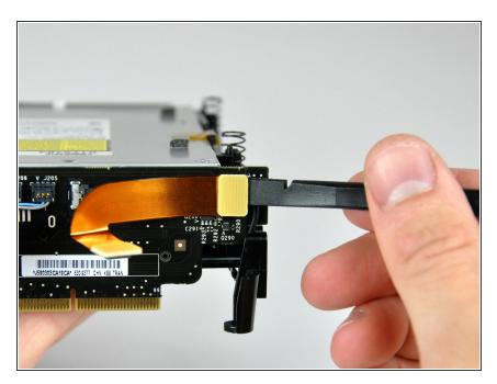
Use the flat end of a spudger to disconnect the audio ribbon cable from the interconnect board.
