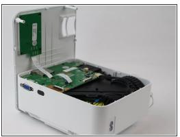
Flip the device over and pry the top off with a plastic opening tool.
