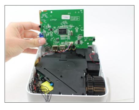
Raise motherboard by lifting sideways and then up to avoid the ports.
