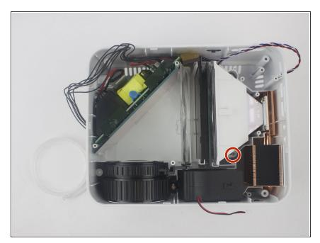
Remove the two screws attached to the lamp with a J0 screwdriver.
