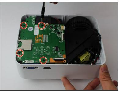
Remove four (6 mm) screws connecting the motherboard using a J0 screwdriver.
