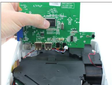
Remove wires attaching the piezoelectric speakers to the motherboard.
