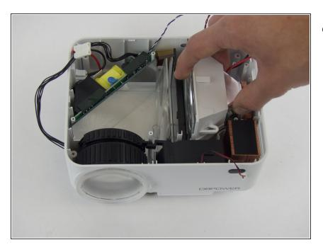
Lift upwards to remove the lamp.
