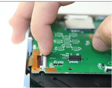
• Lift the black latch on the ZIF connector and remove the ribbon cable that attaches the digitizer to the motherboard.
