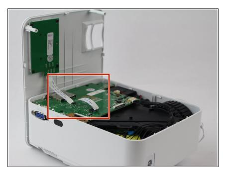
Remove the ribbon cable connecting the motherboard to the button control board by gently pulling it from its connector.
