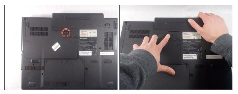
• Slide the lock to the right to unlock the battery from the device.
