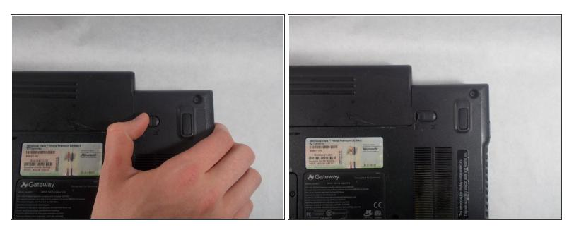
• Put the switch from the locked position to the unlocked position.
