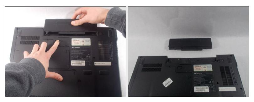
• While holding the 2nd lock in the unlocked position, pull the battery away from the laptop.
