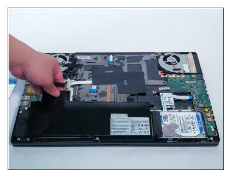
• Lift the battery and remove.
