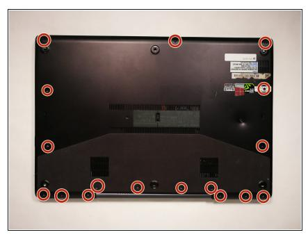
Remove all screws using the JIS #1 screwdriver.
