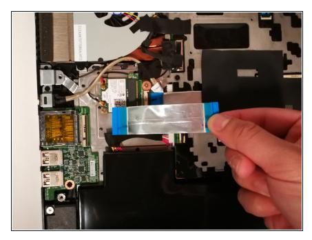
Remove the foil connector by pulling on the blue tabs.
