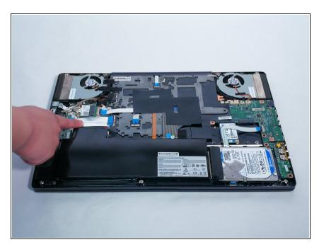
• Locate the foil connector above the battery.
