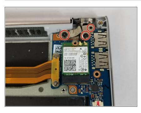
Remove the three Phillips #00 screws securing the hinge to the IO board.
