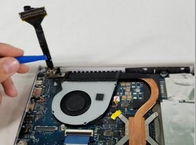
Remove cable connecting the screen assembly to the the motherboard.
