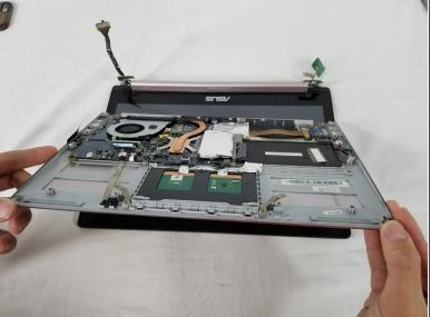
Lift the entire lower assembly up and off of the hinges securing it into place.
