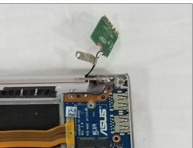
Remove the Wi-Fi card by pulling it straight out of its connector.
