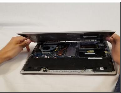
Using a plastic opening tool pry the back panel off of the laptop.
