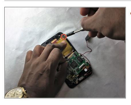
Peeling back yellow tape, remove the 2.5 mm Phillips #0 screws on top of motherboard.
