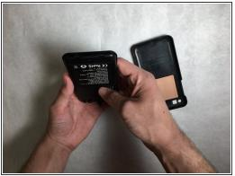
Pull on the indentation and take off the casing of the device.
