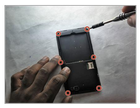
Remove the six 2.4 mm, Phillips #0 screws circled in the image.
