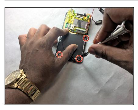
Remove the three 2.5 mm Phillips #0 screws attaching screen to main assembly.
