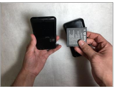
Remove the faulty battery and insert a replacement in its slot.
