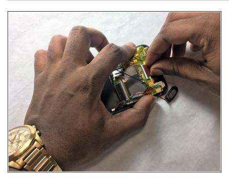
Remove ribbon cable on top of motherboard.
