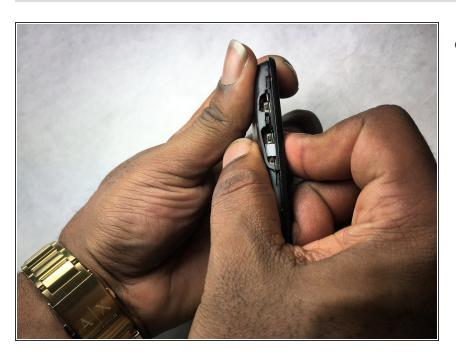
Remove inner casing exposing the motherboard.
