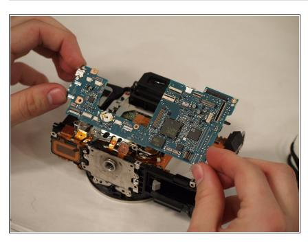
Remove the motherboard from the device.
