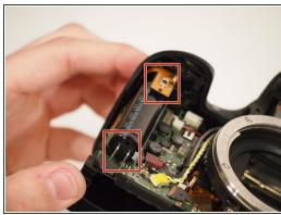
Using the plastic opening tool, pry the front of the casing off of the camera.
