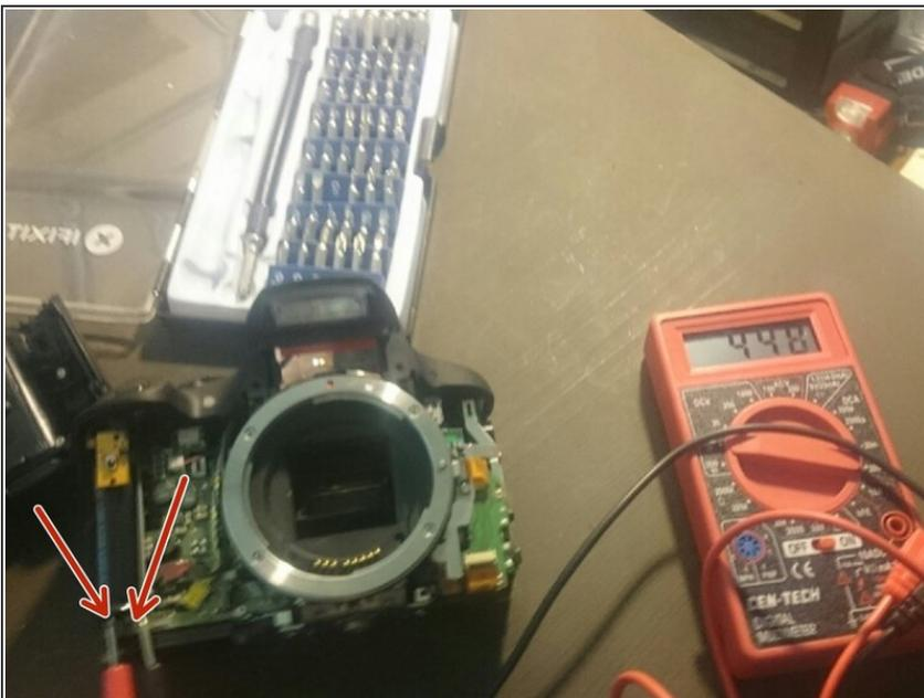
ⓘ The meter will fluctuate with a current until reaching zero. This process will discharge any residual charge.
