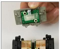
• Lift the mic connector from the base of the device and replace with a new component.
