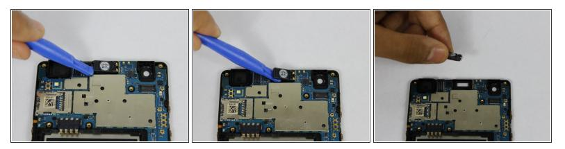
• Using a plastic opening tool, pry up the front facing speaker and remove it from the phone.
