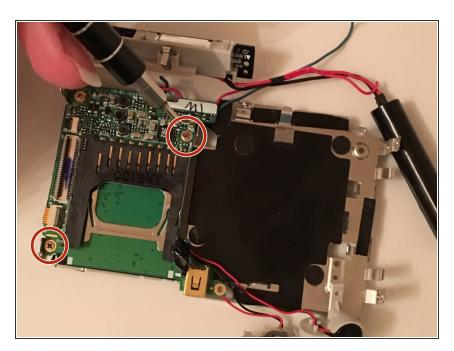
Remove the two Phillips #000 screws securing the motherboard.
