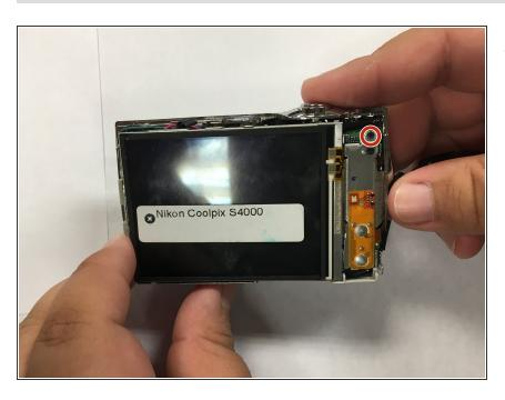
Remove the single 3mm Phillips #000 screw from the back of the camera.
