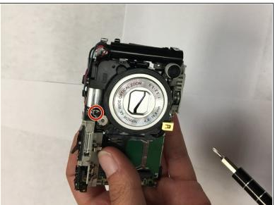
Remove the two 3mm Phillips #000 screws.
