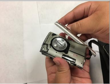
• Use your fingers, or a spudger, to lift up one end of the casing and then pry the two pieces apart.
