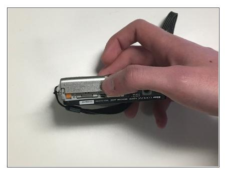
Slide the battery door open with a finger or thumb and release it so the door opens.
