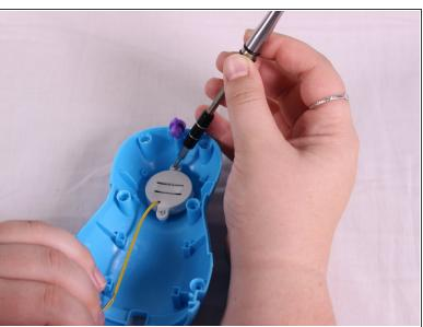
Remove the two 7mm Philips #00 screws from the head.
