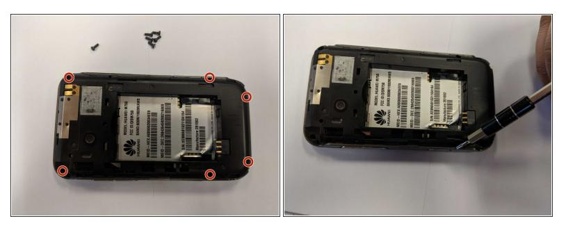
Using the T5 Torx screwdriver, remove the six 6mm screws.
