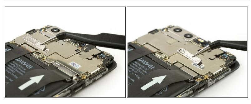
Use tweezers to remove the two cable brackets.
