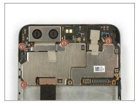
Remove the four Phillips #00 screws from the motherboard.
