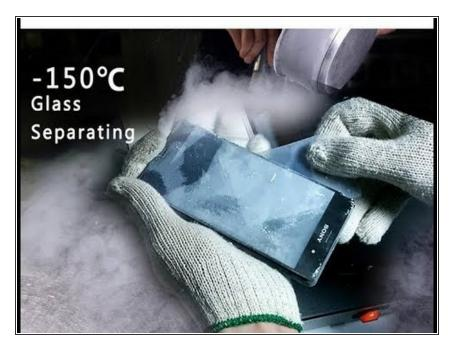
This technique will show you how to replace cracked glass in XPERIA Z3 model with method based on the low temperature. Post your questions in the comments!
