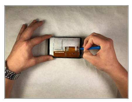
Use a plastic opening tool to loosen the two clips on the short sides of the Nuvi screen encasing to a position that allows the removal of the screen.
