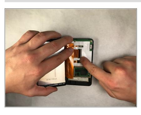
Once the body of the n\u00fcvi is separated, carefully flip the tabs on the motherboard that secure the ribbon cable to the motherboard and disconnect.
