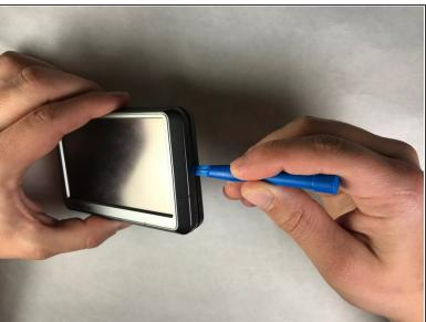
Once the screws are removed, use the plastic opening tool to carefully separate the body from the screen encasing.
