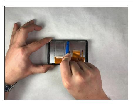
Use a plastic opening tool to loosen the three clips located on the top of the screen encasing to a position that loosens the hold on the screen.
