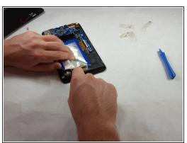
Remove the three pieces of adhesive placed over the edges of the battery.
