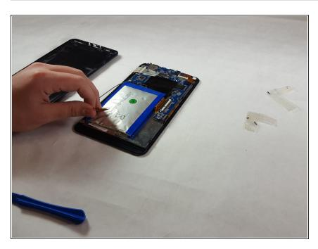
Remove the wifi antenna from the bottom of the battery.
