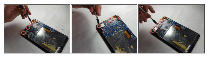
Remove the three 2.5 mm Phillips #1 screws holding the motherboard to the case.
