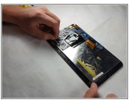
Remove 3 ribbon cables attached to the motherboard by lifting the plastic retainer, then pulling the cable out.
