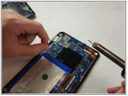
Heat up the soldering iron, proceed to desolder and remove the battery connections.
