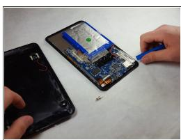
Remove the device's back cover using the plastic opening tool.
