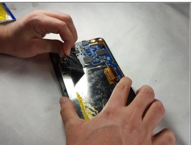
Remove adhesive attaching the motherboard to the casing.
