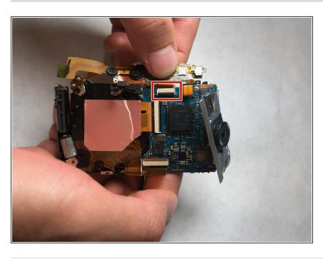
Lift flash component toward you and gently pull the ZIF cable up and away from the camera.
