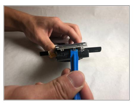
• Working on the left side of the screen, pry the metal panel off from the motherboard housing using a plastic opening tool.
