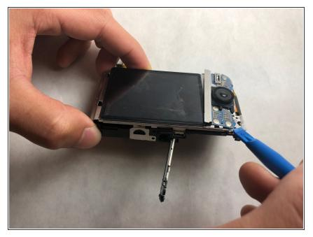
• Pry back the panel to the right of the screen using a plastic opening tool.
