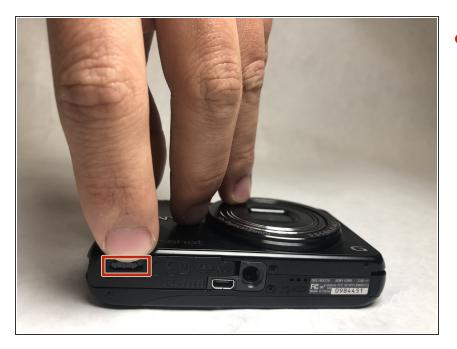
Slide the gray switch from lock to open position.
