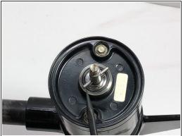
• Remove the drive pin by pushing on either side so it slides out.
