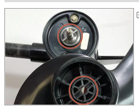
When reinstalling your new propeller, make sure to properly align the drive pin with the base of the new propeller.
