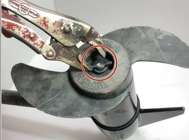
Remove the locking nut by turning in a counterclockwise motion.
