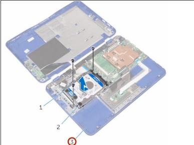
• Slide and lift the hard-drive assembly off the palm rest and keyboard assembly.
