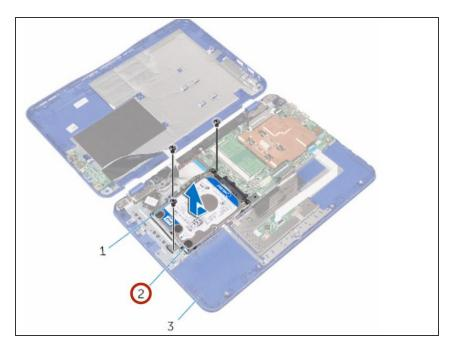
Slide and connect the hard-drive assembly to the connector on the system board.
