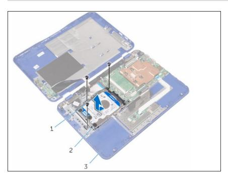
Align the screw holes on the harddrive assembly with the screw holes on the palm rest and keyboard assembly
