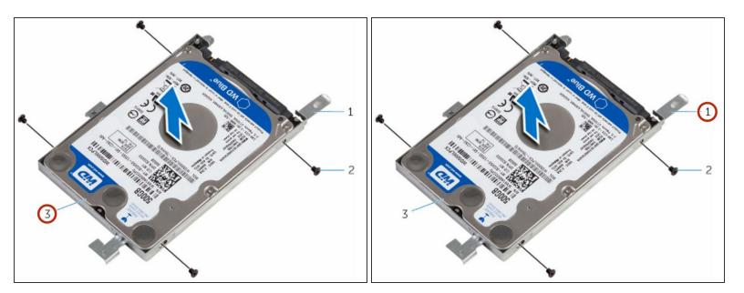
• Lift the hard drive from the hard-drive bracket.
