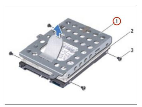
Lift the hard-drive bracket off the hard drive.
