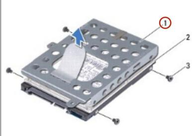
Place the hard drive in the hard-drive bracket.
