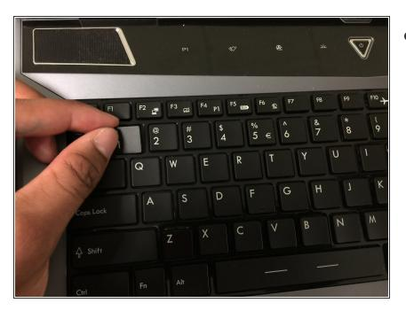
Apply force to the key until all key clips are properly attached.
