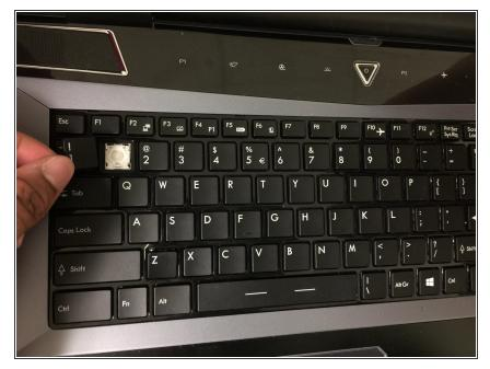
Repeat the previous step on all the keys corners and remove the key from its socket.
