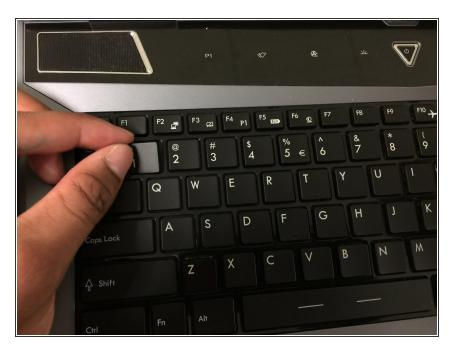
Place your new key in the appropriate slot positioned as if the key was fully functioning.
