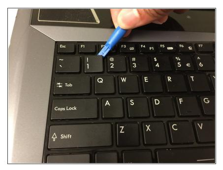
Lift up the corner of your desired key using a spudging tool to create leverage.
