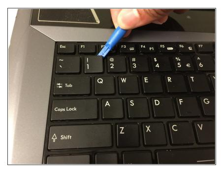
Apply lifting force to the corner until a portion of the inner key clips are detached.
