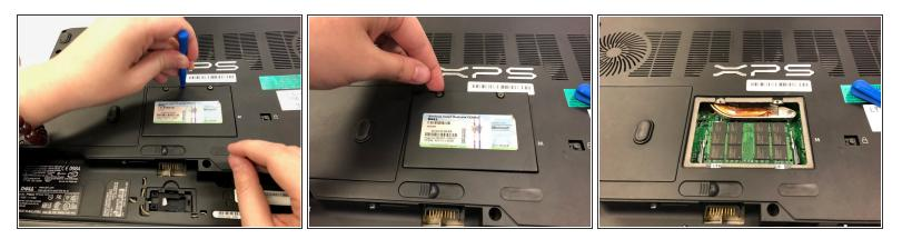
• Use a plastic opening tool to pull up and remove the center panel.
