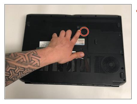
Push the sliding button near the battery compartment.
