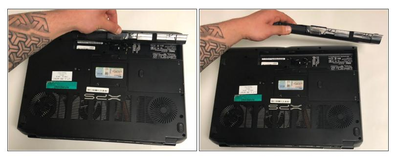
• Lift and remove the battery.
