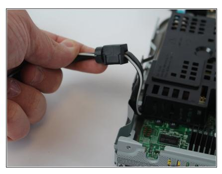
• Lift up the power cord at its base to remove it.
