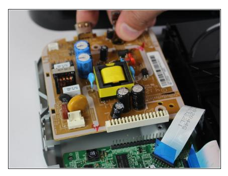
Grip the edges of the motherboard and pull upwards to remove.
