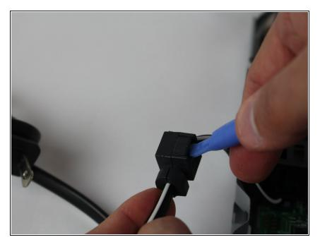
Insert a plastic opening tool into the black plastic tab on the cord and twist to separate.
