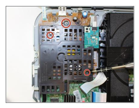
Remove the three screws holding down the cover with a Phillips #0 screwdriver.
