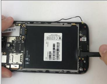
• Use the flat end of a spudger to pry up on the connector at the bottom of the battery space.
