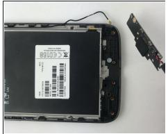
• Insert the tweezers under the vibrator and gently lift up the whole part.
