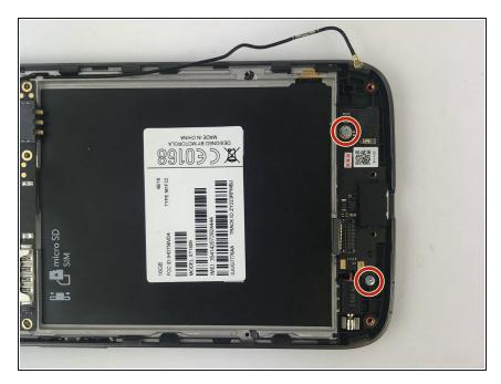
Remove the two (2) 3mm Phillips PH000 screws securing the charging port.
