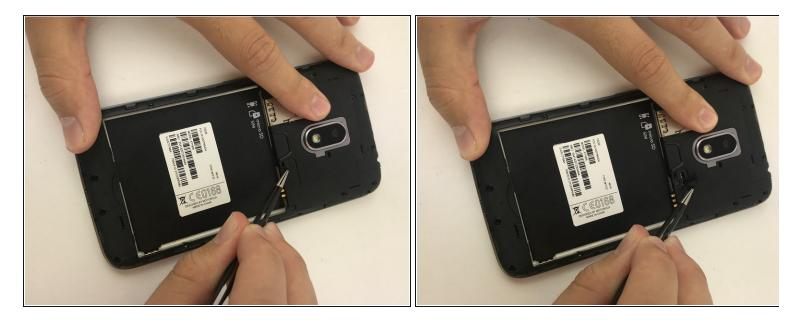
Remove the small silicon cover at the bottom right of the camera using tweezers.
