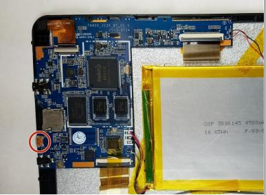
Place the tip of the soldering iron on the four points circled in the image long enough to liquefy the surrounding solder.
