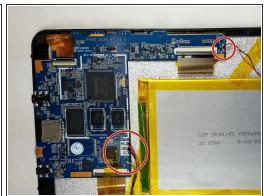
Using a soldering iron, desolder the points circled on the picture until the solder has liquefied enough to be able to remove the wires from the circuit board.
