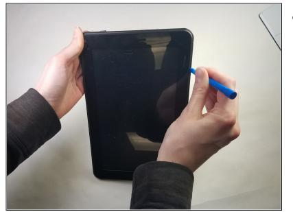
Using the plastic opening tool, insert it into the crease where the glass screen meets the housing of the rest of the tablet. Once inserted, keep inserted and run along the edges to separate the plastic clips from each other to dislodge the back plastic away from the glass and internal components.
