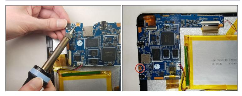
Place the tip of the soldering iron on the four points circled in the image long enough to liquefy the surrounding solder.
