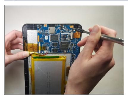
• Using the PH00 screwdriver, unscrew the four 4.4 mm screws that are anchoring the circuit board down to the rest of the tablet.
