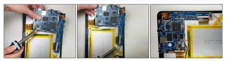
• Using a soldering iron, desolder the points circled on the picture until the solder has liquefied enough to be able to remove the wires from the circuit board.
