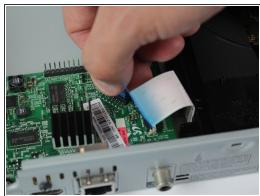
Firmly grip the hard plastic tab attached to the base and pull upwards.
