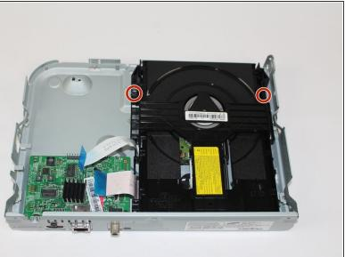
Remove the two 7mm screws with a Phillips #1 screwdriver.
