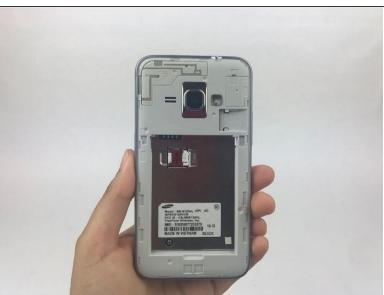
• Locate the notch in the lower right corner of the battery then lift the battery out.
