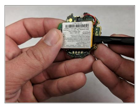
The battery is glued to the motherboard and will need pried off with a nylon spudger.
