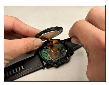
Disconnect this ribbon from the motherboard using tweezers.
