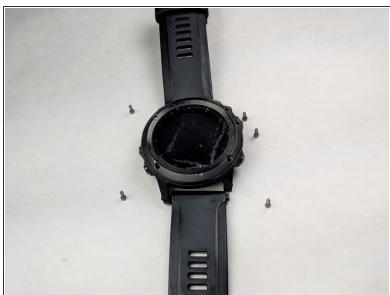
Remove the five 7mm screws with H1.3 hex screwdriver.
