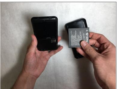
Remove the faulty battery and insert a replacement in its slot.
