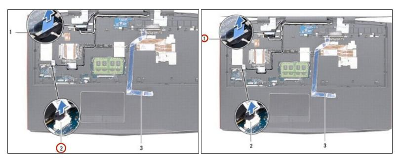
Disconnect the LED-logo board cable from the connector on the system board.
