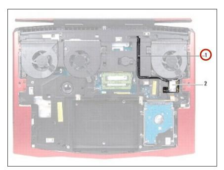
• Slide the Mini-Card antenna cables through the slot on the computer base.
