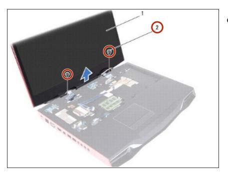
Remove the two screws, on the display hinges, that secure the display assembly to the computer base.
