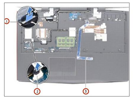
• Connect the display cable, videocard connector cable, and LED-logo board cable to the respective connectors on the system board.
