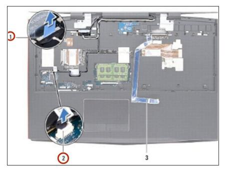
Route the display cable and LED logo board cable through the routing guides on the palm-rest assembly.
