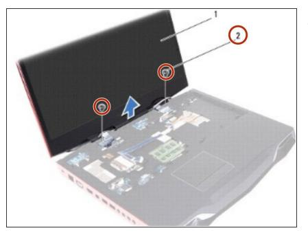
Place the NEW display assembly in position and replace the two screws, on the display hinges, that secure the display assembly to the computer base
