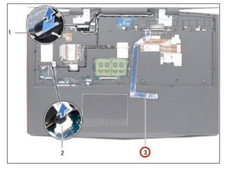
• Disconnect and peel off the videocard connector cable from the connector on the system board.
