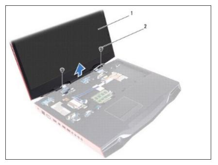
Move the display to a perpendicular position to the computer base, and then lift the display assembly off the computer.
