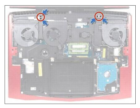
Remove the four screws that secure the display assembly on the computer base.
