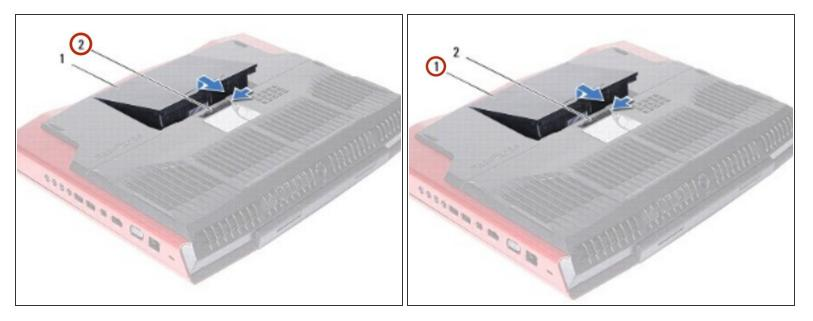
• Slide the battery latch to the unlock position. The battery pack pops up.
