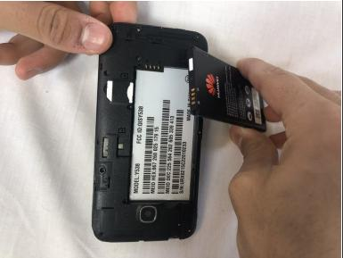
• Use the flat end of a spudger, or fingernail, to lift up the battery and pull out.
