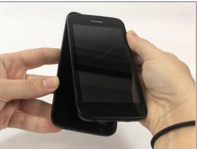
Wedge your thumb nail, or the flat end of a spudger, into the bottom left corner and pry off.
