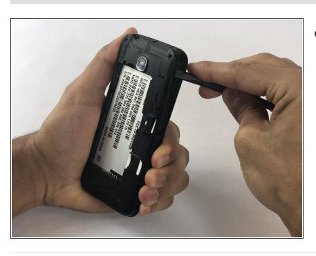
Use the flat end of a spudger to pry off the back panel.
