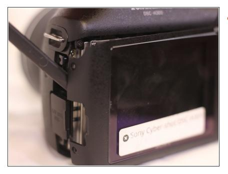
Use the flat end of a plastic spudger to pry apart the rear cover from the body of the camera.
