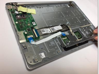
Remove the metal piece that secures the trackpad cover in place using the opening tool.
