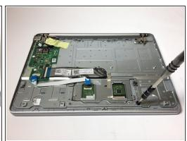
• Remove the 4, 2.5 mm screws from the trackpad cover.
