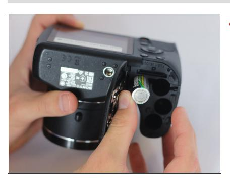
Remove the batteries.
