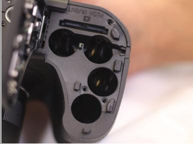
Place thumb on battery cover and slide outward until it springs open.
