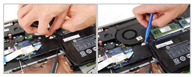
• Disconnect the fan cable by pulling it out of the motherboard socket.
