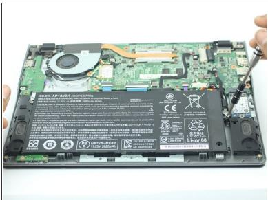
Remove the two 3.6 mm Phillips screws holding the battery in place.
