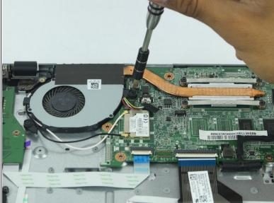
Remove the six 4.7 mm Phillips screws that secure the fan.
