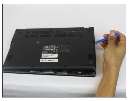
Use the plastic opening tool to carefully remove the bottom.
