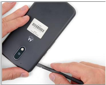
Slide your tool all along the side of the phone to separate more of the clips securing the back cover.
