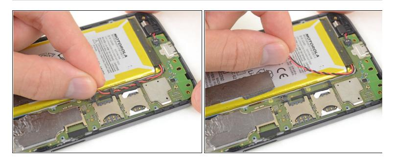
• Push the battery wires towards the battery to de-route them from the black bracket on the motherboard.
