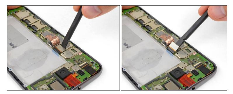
• Use your spudger to disconnect the display by prying its connector straight up from the motherboard, on the edge nearest the side of the phone.
