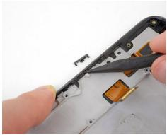
• Push the power button out of the frame from the inside by carefully pressing the tip of your spudger against the tops of the two mushroom pins securing it.
