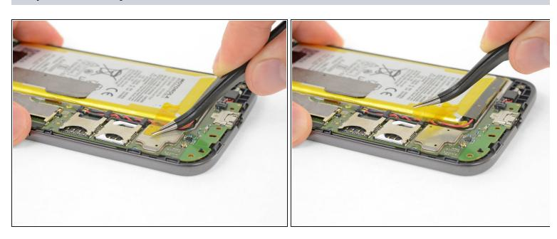
• Peel up and remove any tape connecting the battery to the main board.
