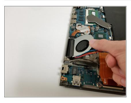
Lift the internal cooling fan to remove the fan from the device
