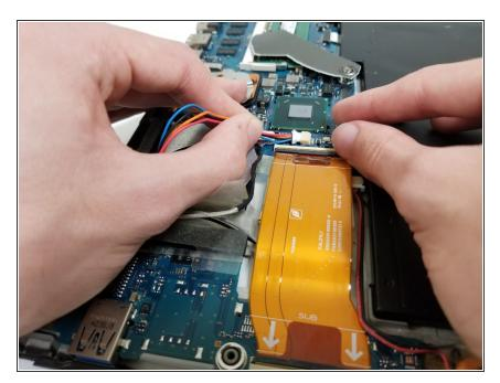
Unplug the internal cooling fan by tugging gently on the wire attatched to the device's motherboard
