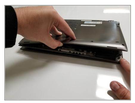
Peel off hard cover to expose interior of device
