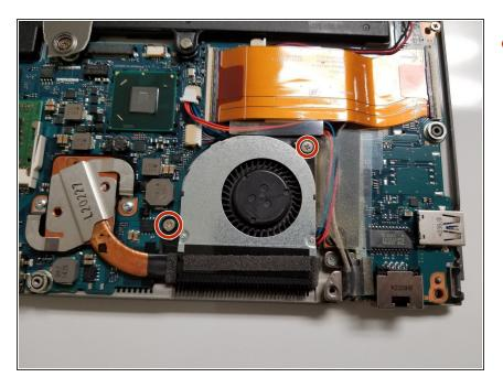
Remove the two 1 mm screws using a Phillips #2 screwdriver.
