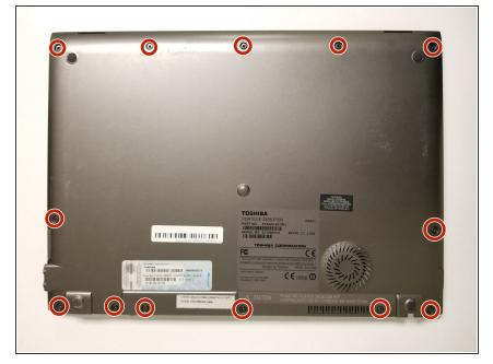
Remove the thirteen 1.4mm screws on back of device using a Phillips #2 screwdriver.
