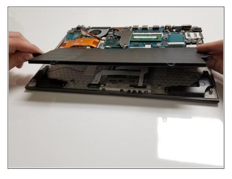
Lift battery up by its sides, and it should easily come off.
