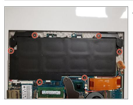
Remove the six 1 mm screws using a Phillips #1 screwdriver.
