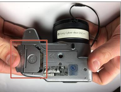
Push down on the grey arrow (pointing left) and slide left (while holding the grey arrow down).
