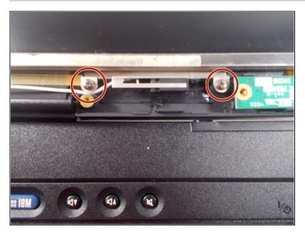
Remove the two screws located near the bottom middle of the screen
