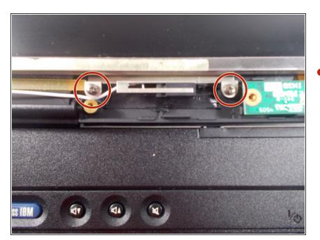
Remove the two screws located near the bottom middle of the screen
