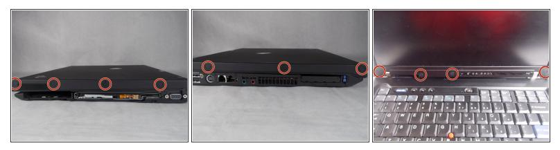
• Locate the screws holding the screen cover in place.
